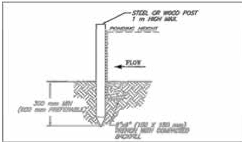
Figure 4. Proper installation of sediment fencing
